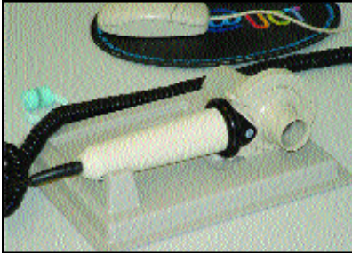
Fig. 2. A modern unheated pressure-drop pneumotachograph which requires only attachment to a personal computer loaded with the appropriate software.
