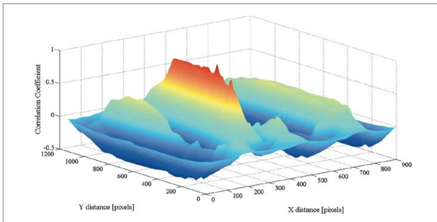
Fig. 2. A cross-correlation plot of two 2D images. The peak in red indicates the XY position at which the images have the best alignment.
