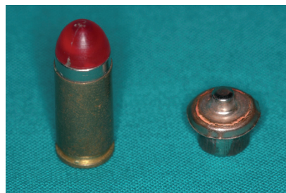
Fig 4(b). The Eliminator projectile has a small plastic cap which covers a central pillar, and which may cause a second skin wound at close range. Note the flattened shape of the spent projectile, meaning more effective energy transfer to the tissues.
