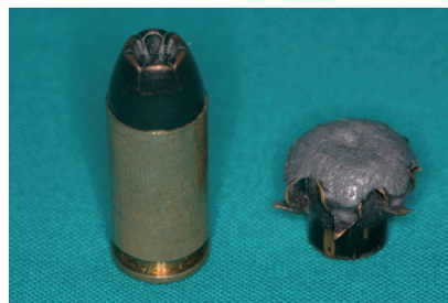
Fig 4(a). The Black Talon projectile, with exceedingly sharp edges that are folded open upon impact, may cause severe tissue destruction – and injure the unwitting surgeon!
